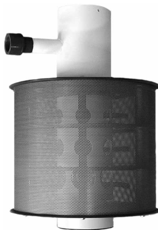
Perforated Stainless Screen .117" Perf. 16GA 316SS
